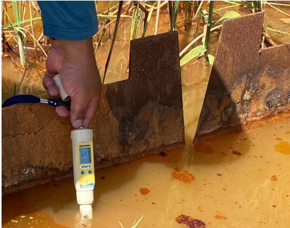
Figure 7 – Seep 1A – pH 6.47 at the V-notch weir (the discharge point) on 08/14/24 (view northwest, 08/14/24)
